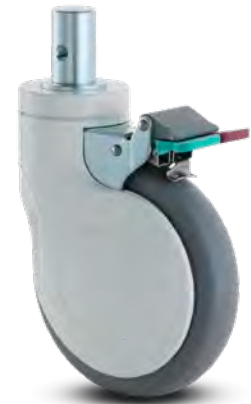
Combo Direction/Total Lock design features two locking pedals that allow separate control of wheel and steering lock. Off pedal unlocks both simultaneously.
